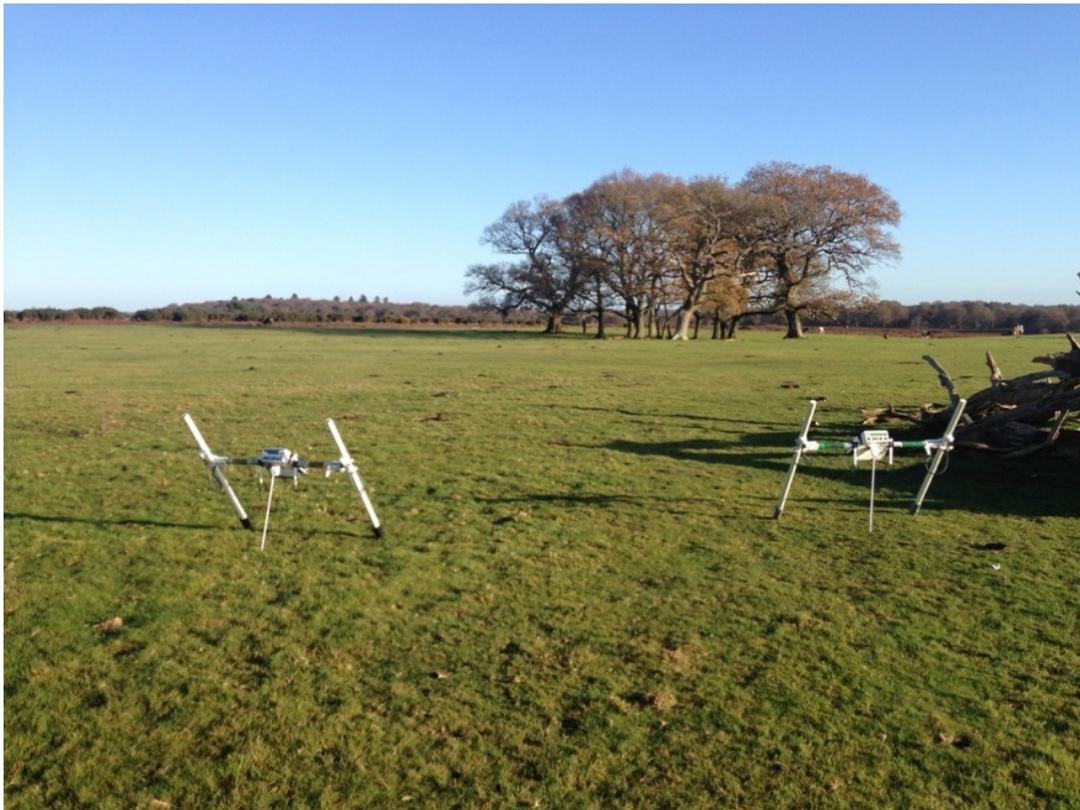
It was a fantastic opportunity for an amateur to use state of the art equipment such as the magnetometers as shown here. The key to the surveying technique is to hold them at arms-length and walk at a steady pace over rough ground and through foliage! You can’t wear any metal eg zips or buckles, and it is harder than you would think!
